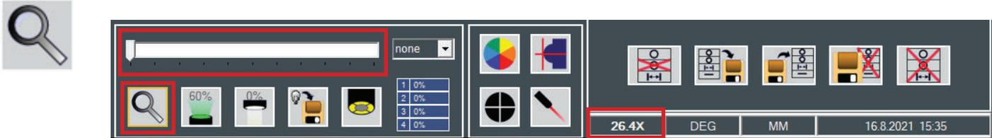
The magnification value appears within the screen area to the system parameters. This value matches the true magnification between the part and the video image (the size of the screen may affect the chosen value).
