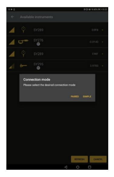
It may arrive that the connection fails. In that case the application will automatically try to reconnect your instrument for 2 minutes.
