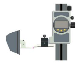
Maximum permissible error widthwise: 0.01 mm
