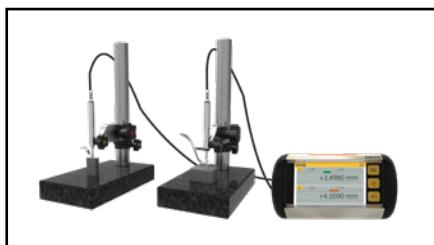
2 probes P12D connected to a D62S.
