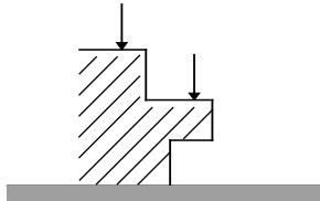
Use the UP/DOWN button on the back of the instrument to move the motorised carriage until the measurement probe is in contact with the base surface (surface table). Press the SET key to have the zero or preset origin set on this position.
