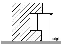
Use UP & DOWN button on the back to move the probe UP and DOWN, until the probe is on contact with the first surface.
