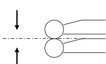
Press the CST key and touch one of the ground surfaces of the cylindrical gauge. Release the probe and touch the opposite surface. The probe constant value is displayed and memorized until a new constant value is taken. The value of the constant is stored and then displayed for a few seconds.
