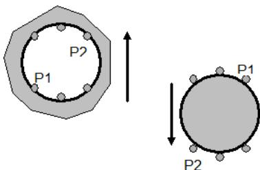
1. Move the probe inside of the bore (or onto one side of the shaft) using up & Down button on the back and start measuring at a point P1 which is well away from the summit of the curve
