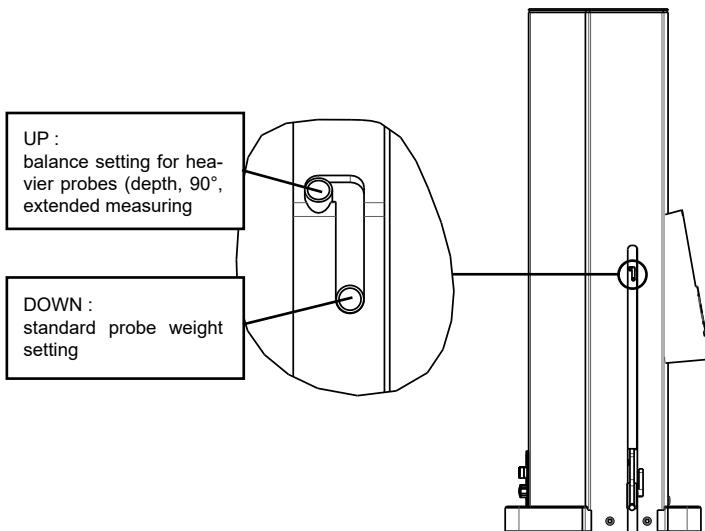
The weight adjustment selector enables with a screwdriver 00 or a pen.
