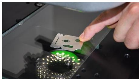
6 Move Z-axis until you get a sharp image, and set the light sources for optimum edge detection.
